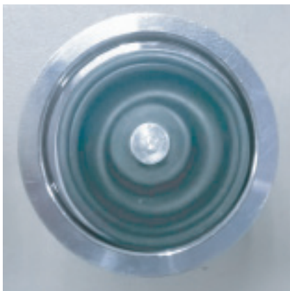
Figure 9 - Correct diaphragm alignment
