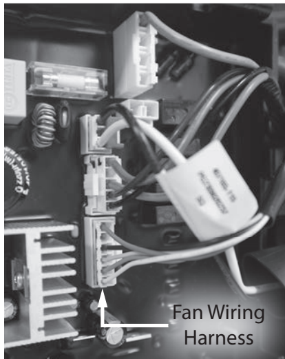
Figure 95 - Locate fan wiring harness on control board
